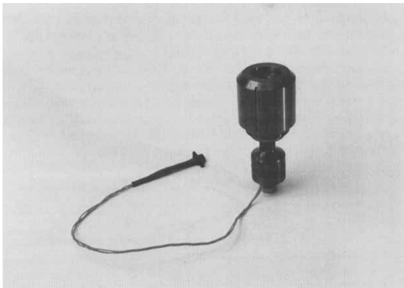
FIGURE 1 The clamp pressure cell made of maraging steel ( \phi_{\text{inner}} = 8 mm, \phi_{\text{outer}} = 48 mm at sample level).
